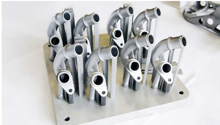
Sample metal 3D printed water connectors for the Audi W12 engine. Photo via Volkswagen AG
